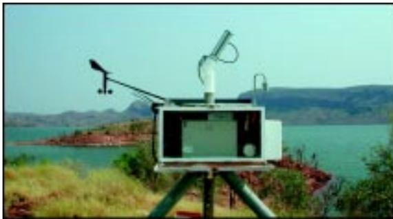
The Lake Argyle ground station was first installed in May 1999 and tested at three different locations (including South Pelican Island as shown here) before being set up near the museum in October 2001. The sun photometer is mounted on top of the apparatus for a clear view. The twin collimators reminiscent of shotgun barrels are used to reduce stray light entering the instrument.
